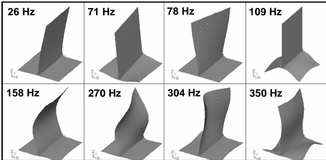
Figure 2: Typical Mode Shapes for the Test Structure.
